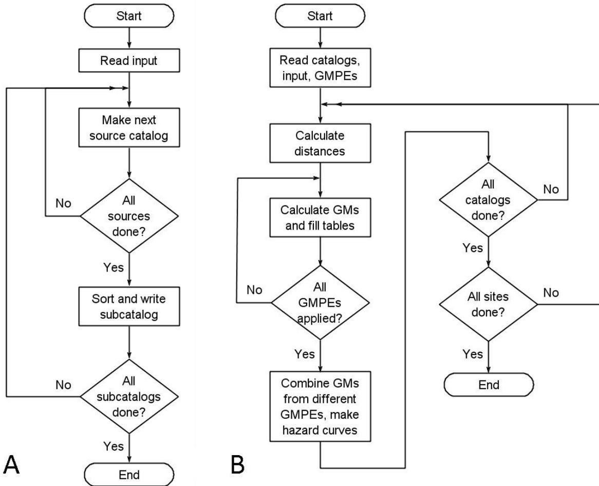
Figure 1. A) Flowchart of program EqHaz1; B) Flowchart of program EqHaz2; input to EqHaz2 is the output from EqHaz1.
