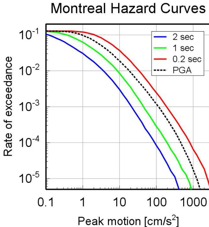
*Figure 4 – Plot of mean-hazard curves constructed by EqHaz2 for the example application in Montreal. Ground-motion amplitudes are plotted for horizontal-component pseudo-acceleration, for a reference site condition, for periods of 0.2, 1 and 2 sec, and peak ground acceleration (PGA).*
