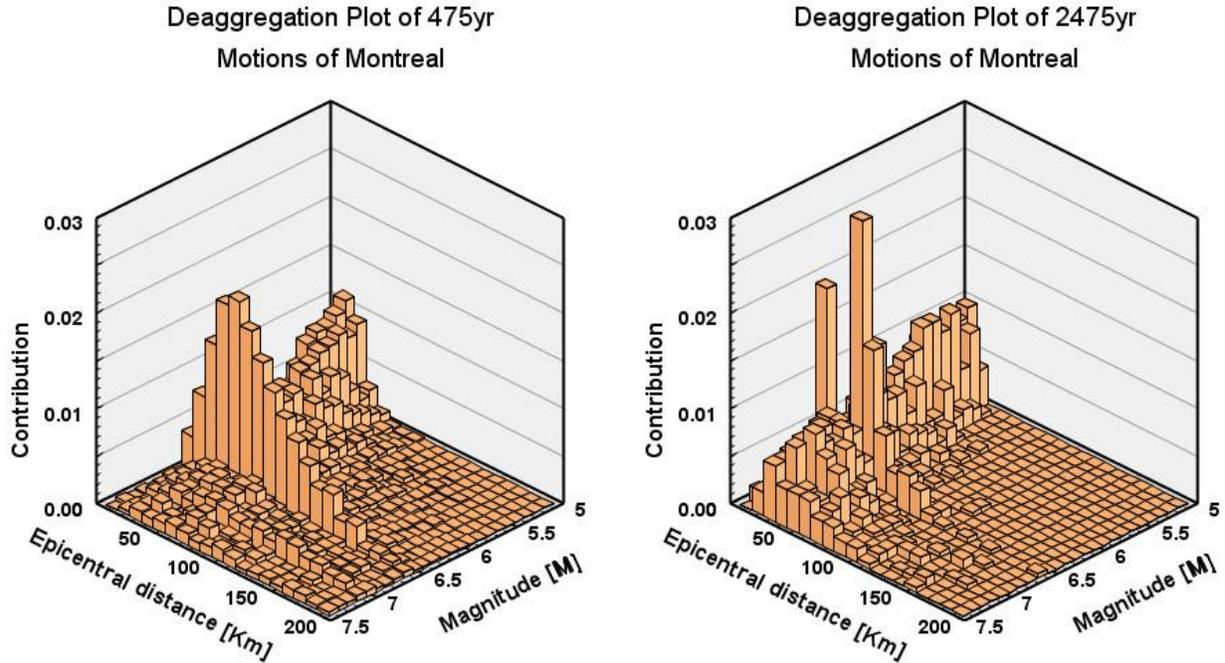
Figure 6. Contributions of different magnitude-distance bins to the  $T=0.2\text{sec}$  PSA hazard in Montreal, calculated from a 4.95Myr synthetic catalogue.
