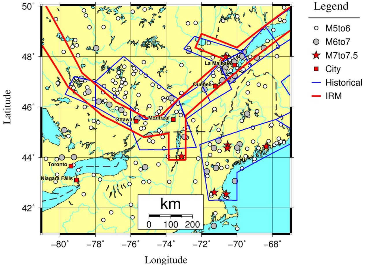
Figure 2 – Source zone boundaries of historical seismicity zones (blue lines;  $M \leq 6.5$ ) and overlying characteristic IRM zone (red lines:  $M 6.5$  to  $7.5$ ), along with a 2475 year subcatalogue of events of  $M \geq 5$  generated by EqHaz1. Events outside the source zones come from a prescribed “background” seismicity rate. Example hazard calculations will be performed at Montreal.
