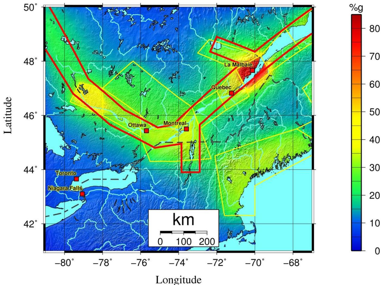
Figure 3 – A sample 1/2475 per annum mean-hazard map of PSA( $T=0.2s$ ) based on the Atkinson and Goda 2011 source model for eastern Canada(as shown in Figure 1).
