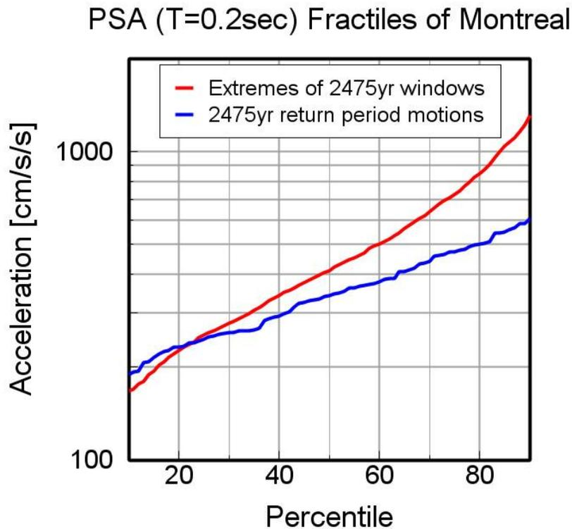
*Figure 5 – Fractiles for the 2475-year return period motions for PSA(T=0.2s) at Montreal, comparing the amplitudes calculated using the traditional separation of aleatory and epistemic uncertainty (blue line), and the approach in which fractiles of extreme values in 2475-year windows are calculated (mixing epistemic and aleatory variability; red line). These results are derived from a 4.95Myr synthetic catalog based on the Atkinson and Goda (2011) model for*
